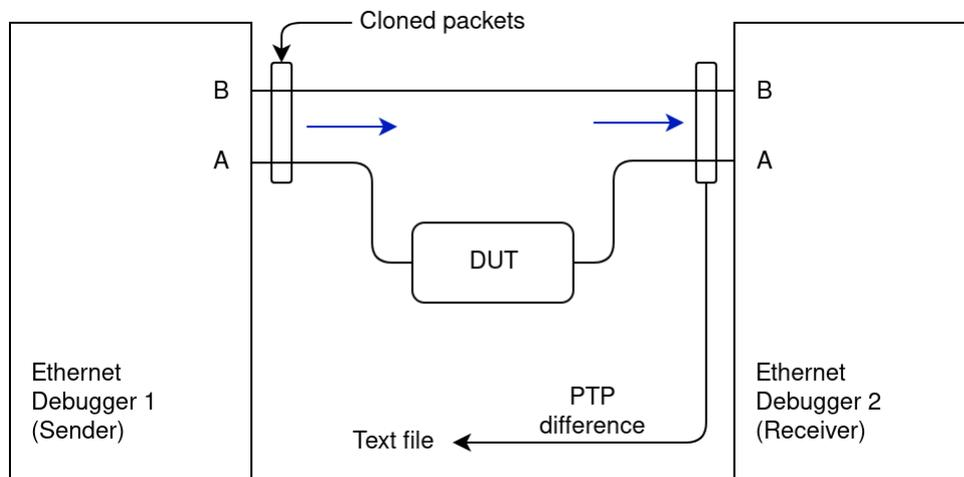
Ethernet Debugger 1 is the sender, Ethernet Debugger 2 is the receiver. The sender generates packets that get sent out of port A and B at the same time. DUT is expected to propagate the packet unchanged to the receiver. The receiver measures the difference in arrival time between port A and B.
